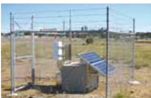
Traditionally, dust monitoring at coal handling facilities has been achieved using dust deposition gauges or stand alone monitors. A major disadvantage of these systems is that data is up to date only occasionally. With environmental management becoming increasingly important, it is vital that monitoring systems can provide near real time information to support the operational and environmental objectives.
