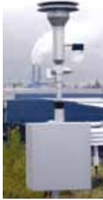
The Beta Gauge type of particle sampler (PM10 or PM2.5) uses a low energy Carbon-14 source to produce a constant source of beta electrons, measured by a Geiger Muller tube or photodiode array. A clean filter tape is placed between the source and the detector and is measured. The tape is then exposed to the air sample before being moved back to the beta source and measured by the beta detector. The difference in beta emissions is proportional to the mass of particles on the tape.
