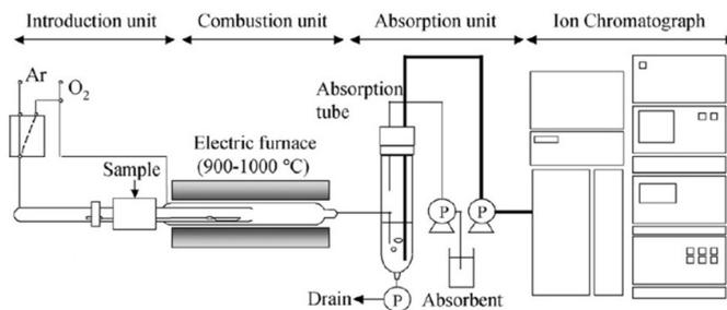
Schematic illustration of combustion ion chromatograph for fluorine (CIC-F).
