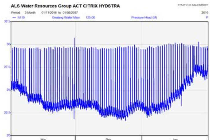
Figure 2. The plot demonstrates baseline water pressure in an ACT suburb. It is influenced by residential water demand and the local feeder reservoir's level. The minor spikes in this trace are from operational changes made by the Water Utility.
