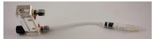
Rotameter and Calibration Tube
