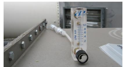
Figure D: Flow is marked by small metal ball. To decrease flow, turn black dial clockwise.
