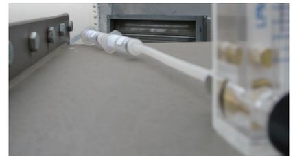
Figure B: Sampling arrows should point toward rotameter. Please note that these figures show two tubes in series. You will only be receiving one tube.
