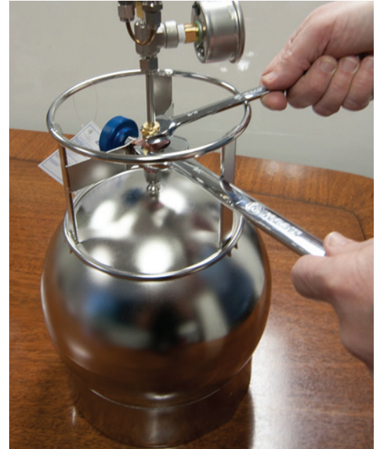
Proper use of wrenches to tighten fittings
