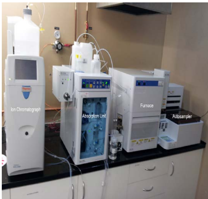
Figure 1. Fully Assembled APH-IC System.
