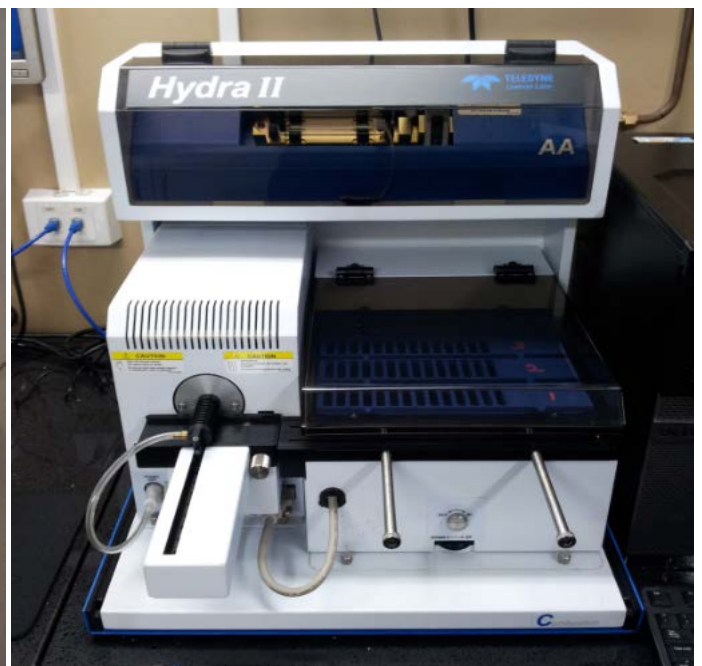
Figure 2. Hydra IIc Automated Mercury Analyser.
