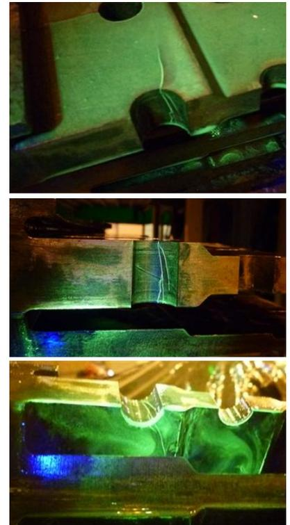
Figure 5 - Cracking to outlet side leg enhanced by FMPI
