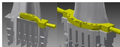
Figure 3 - Bespoke positioning jigs
