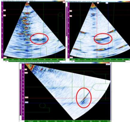
Figure 4 - Phased array images of root finger crack
