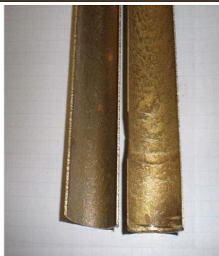
Al Brass tube - inlet erosion
