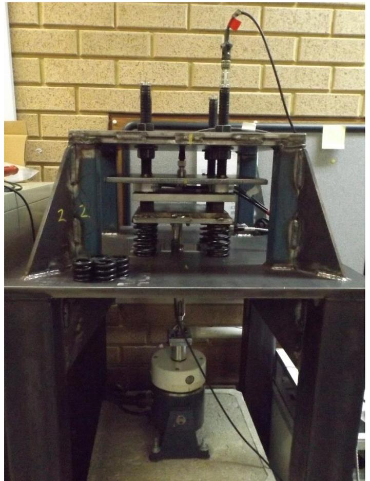
Figure 4 - Test Rig for the Measurement of Dynamic Stiffness
