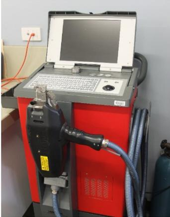
*Spectro mobile arc spark spectrometer*
