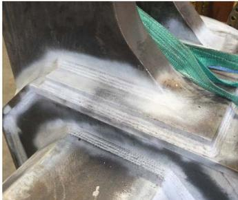
*Mag particle testing of high stress welds*
